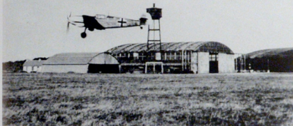
LEFT: This photograph illustrates the uneven retraction cycle of the main undercarriage of a Bf 109 E-4 of JG 2 as it takes off from Cherbourg-Théville during mid-August.
