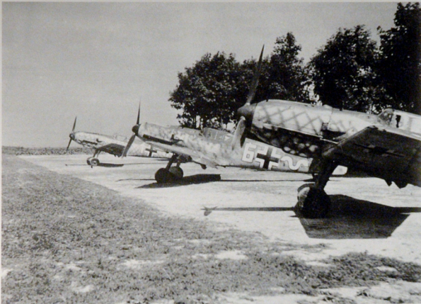
ABOVE: BF 109s of 9./JG 52 at Coquelles, near Calais, early September. While Yellow 6 carried a conventional style fuselage mottle, the other two aircraft have been toned down with the cross-hatch overspray more usually associated with JG 54. As both units were based at Coquelles airfield, it is possible that the common camouflage scheme results from shared workshop facilities.
