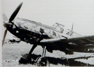
ABOVE: Oblt. Hans Philipp's 'White 1' clearly showing the sprayed cross-hatch finish used to tone down the blue fuselage sides.
