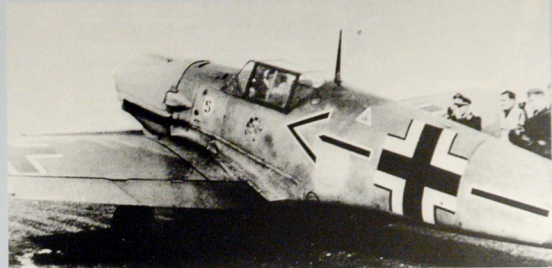
ABOVE: Major Galland's Bf 109 E-4/N, W.Nr. 5819, possibly photographed at Le Touquet in 1941. The fresh paint beneath the forward Stab symbols is believed to indicate the recent installation of nitrous oxide equipment to increase engine power.
